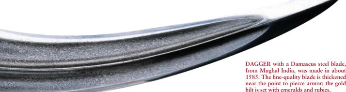
can be found in Indonesia and Japan. The internal structure resulting from these techniques is totally different, though, from that of the wootz blades. To avoid confusion between the two types of manufacture, I refer to the forgewelded blades as "welded" Damascus and reserve the term "wootz" Damascus for the weapons of interest in this article.
