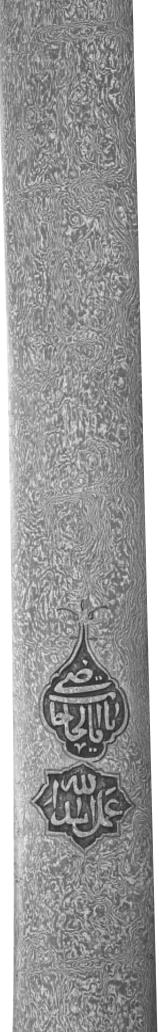
cles that are the lighter bands in the steel. We can show that this lattice is related to the light and dark steel bands in the wootz steel. The distance between dendrite branches is around half a millimeter, and as the ingot is hammered out and its diameter is reduced, this distance is also reduced. The final spacing between dendrites corresponds closely to the distance between bands in Damascus steel.
